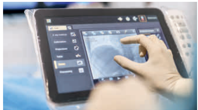
Collimate and pan with a fingertip on the touch screen module Pro
